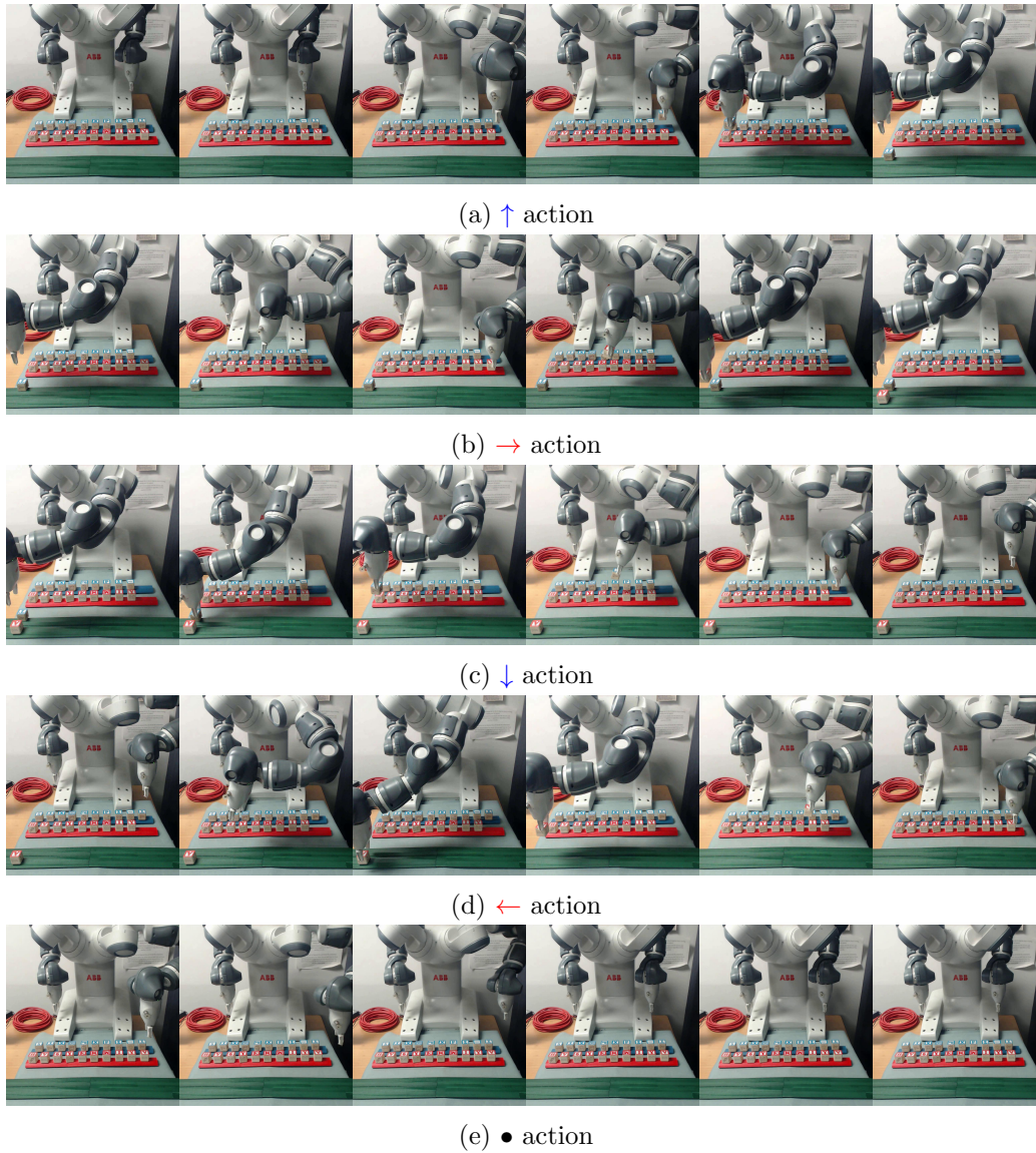
Figure 3: Example trajectories of the robotic arm for each action in the bin packing domain.
