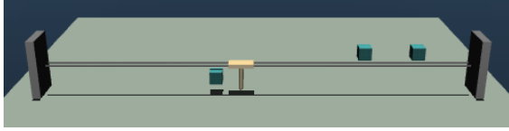
Figure 8: The Rod-and-Block domain. This particular task consists of three obstacles that prevent the rod from moving along the track when the rod is in either the upward or downward position. Different tasks are characterised by different block placements.
